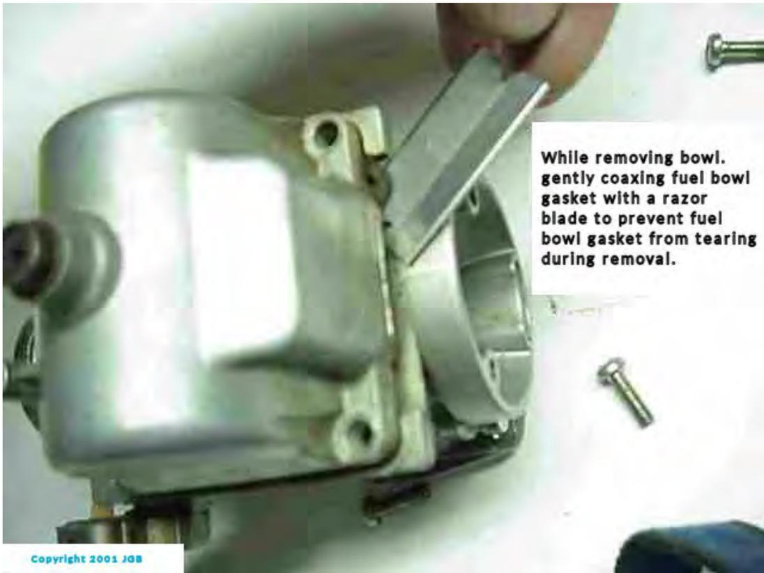
**While removing bowl, gently coaxing fuel bowl gasket with a razor blade to prevent fuel bowl gasket from tearing during removal.**
