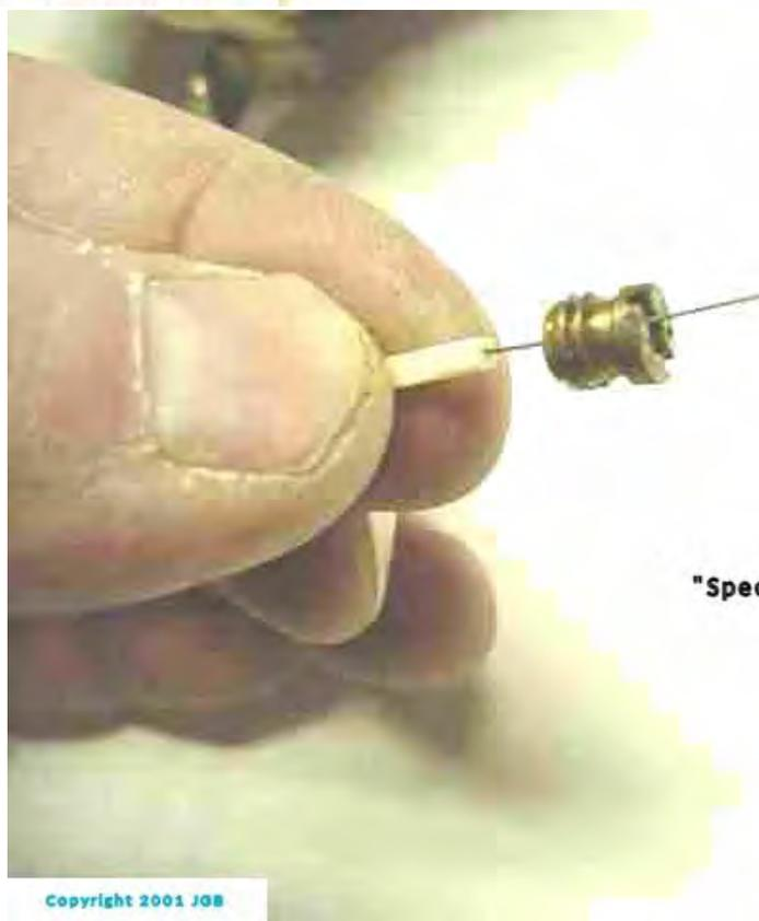
"Special Tool" cleaning Air Jet bore
