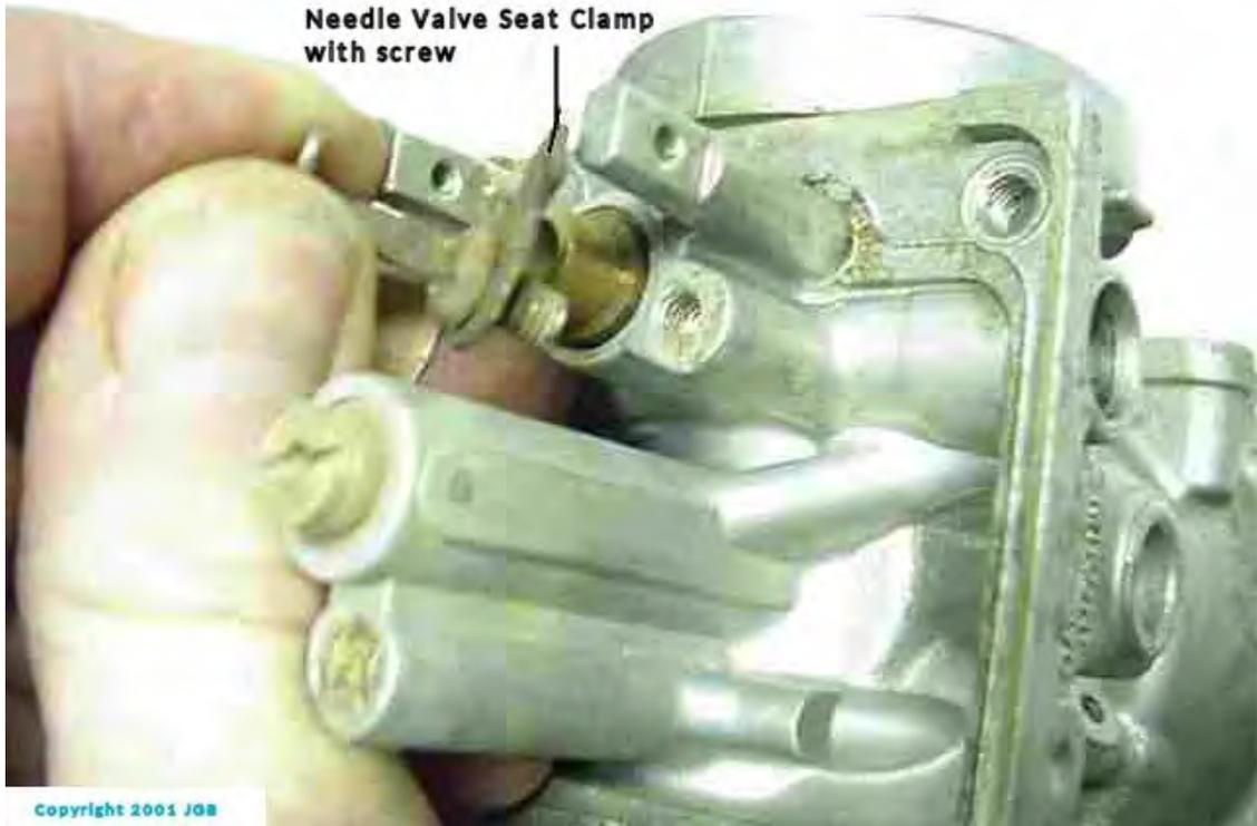
**Needle Valve Seat Clamp with screw**
