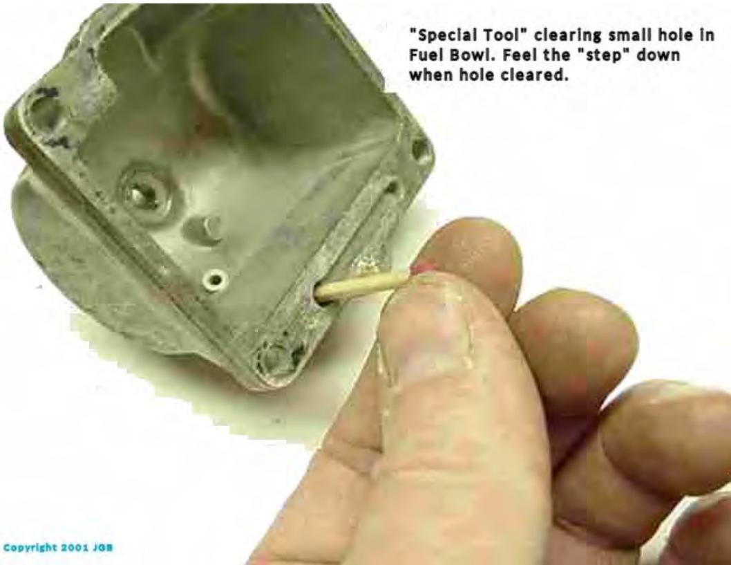
**"Special Tool" clearing small hole in Fuel Bowl. Feel the "step" down when hole cleared.**
