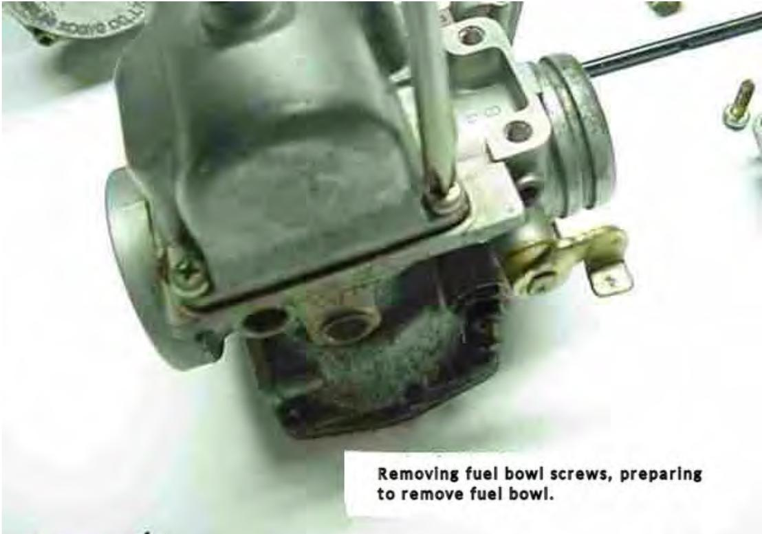
**Removing fuel bowl screws, preparing to remove fuel bowl.**
