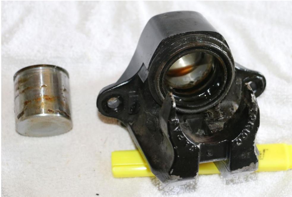
The Piston may be slightly pitted from rust and this is okay, as long as the pits do not run vertically up the side and as long as there aren't too many.
