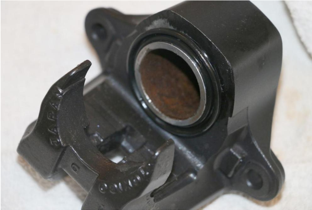
Now you can take this assembly and re-install the Pad Spring. It fits so the rectangular cut out is exactly over the Sight Hole. The tangs should slide down into the sight hole and may or may not hold it in place. You may have to hold it while placing the Caliper Body onto the Caliper Holder.
