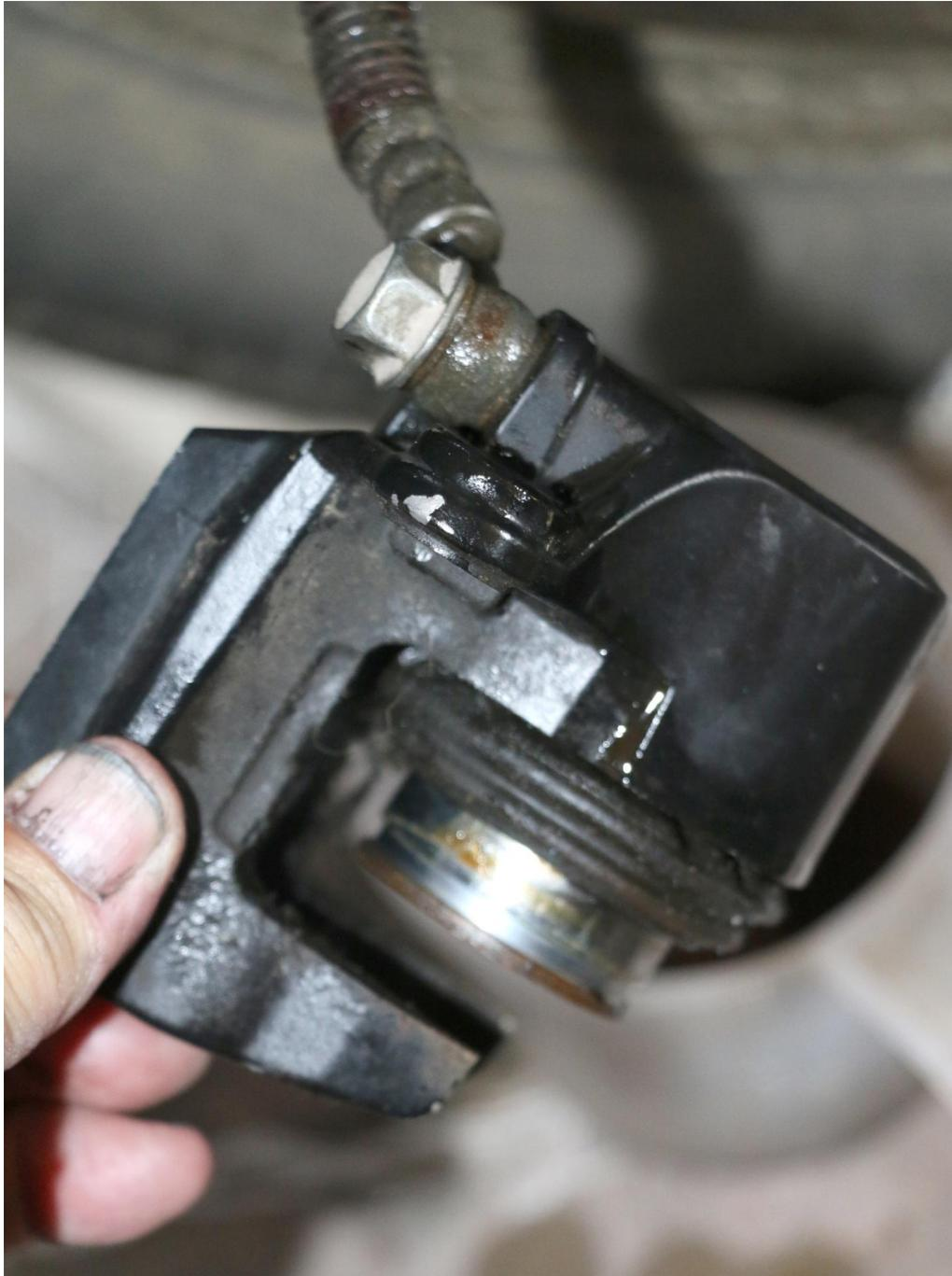
Be aware that you will have to semi-bleed the line first and when the piston releases there will be a fair bit of brake fluid coming out so be prepared to catch it. You should also be aware that brake fluid is a paint stripper so keep plenty of rags on hand and protect painted parts.
