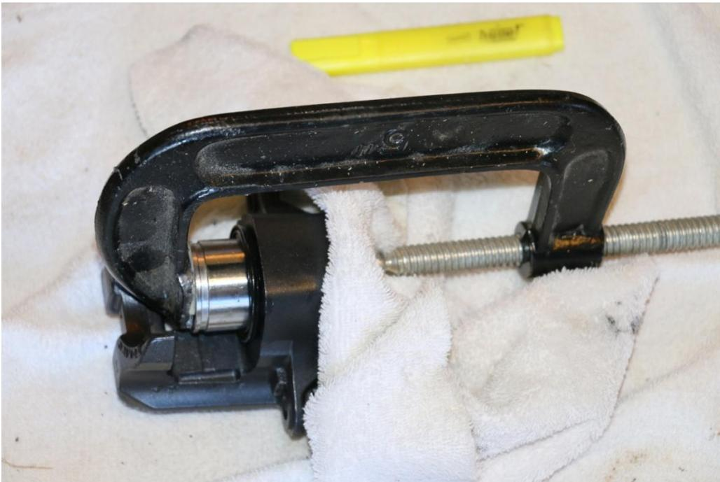
Once the Piston is all the way in the Boot lip will drop into the outer groove on the Piston by itself. But make sure you double check that it has.
