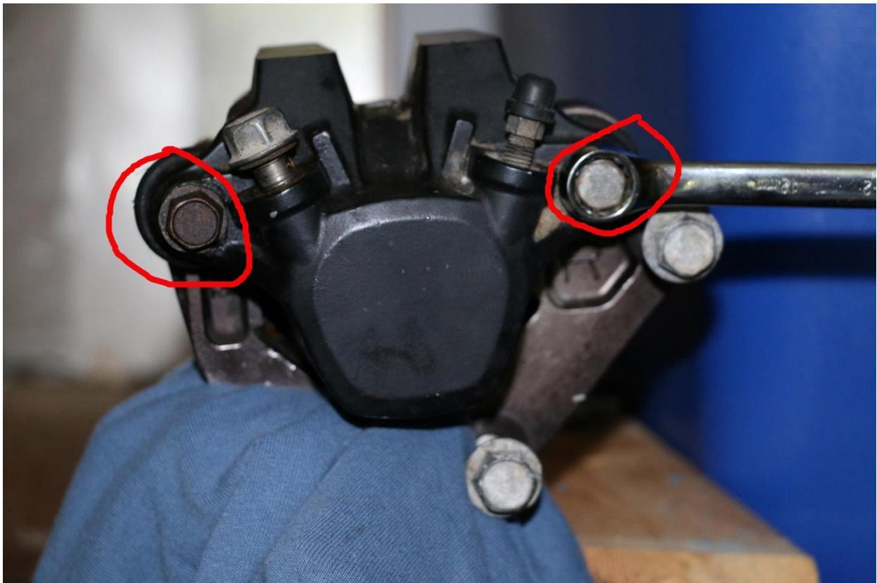
Once these are removed the working part of the caliper will lift off, in fact it may fall off, so be careful.
