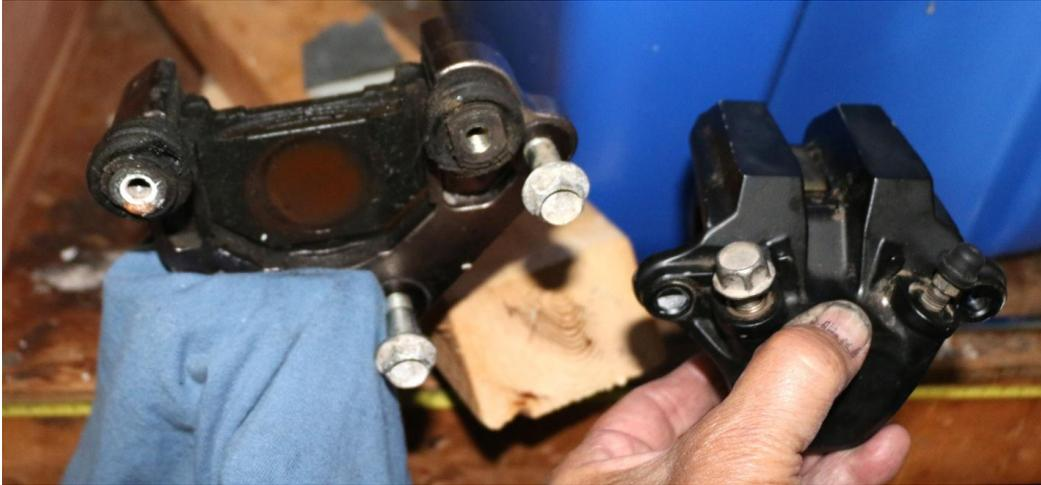
There are several parts in here that are loose once the housing is disconnected – the Pads and the two Pad Guides in the Caliper Holder and, the Pad Spring in the Caliper Body. Ensure you do not lose them.
