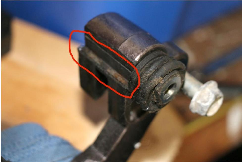
The Pad Spring should also be relatively shiny clean. Again in this caliper the spring was covered in brake dust and road grime that had to be scraped and washed clean.
